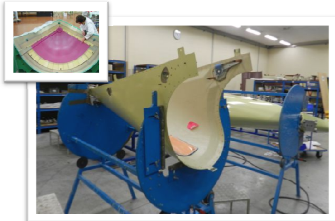
Honeycomb (Flap track fairings A340, A350)
