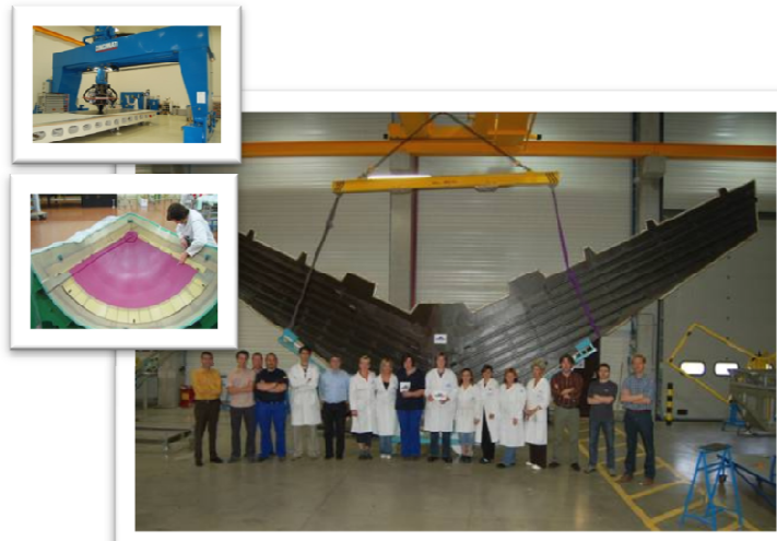
Co cured stringers (HTP Flacon 900/200, SMS, G650)
