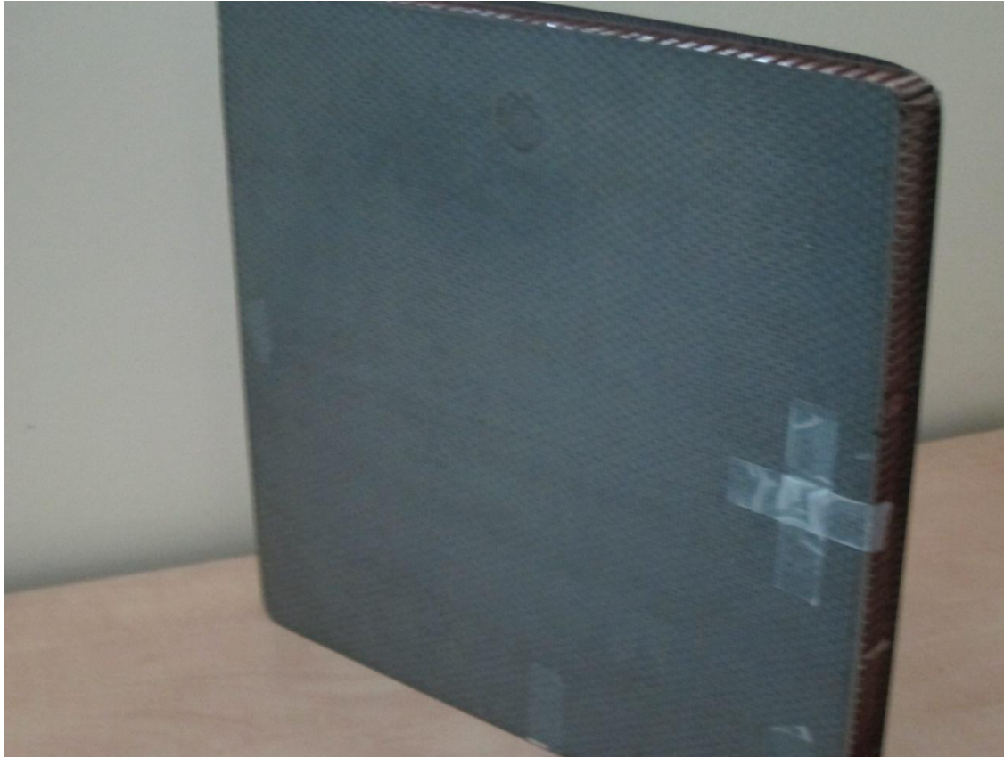
Carbon skin on Honeycomb Structure
