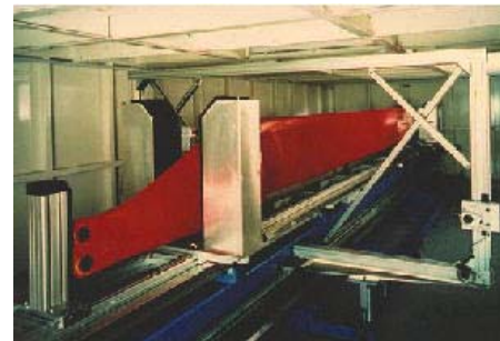
Shearography inspection of helicopter blade Photo: NDT.NET
