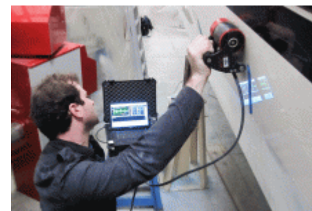
Roller Probe UT Inspection, photo: Sonatest.
